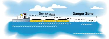
In narrow channels, a tug's or tow's powerful engines can cause a smaller vessel to be pulled toward the tow when passing alongside.
